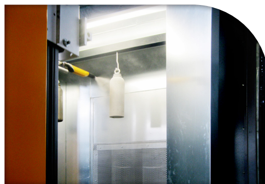
A booth with an automatic powder coating station
