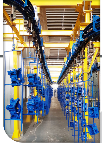
Parts cooling after exiting the curing oven
