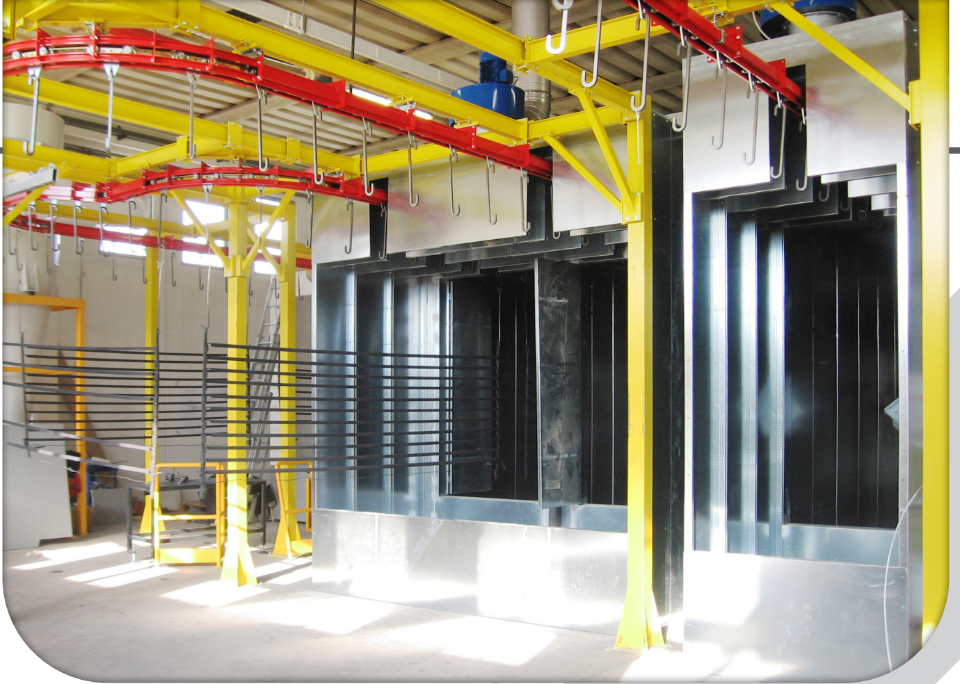
A liquid painting plant's baking oven
