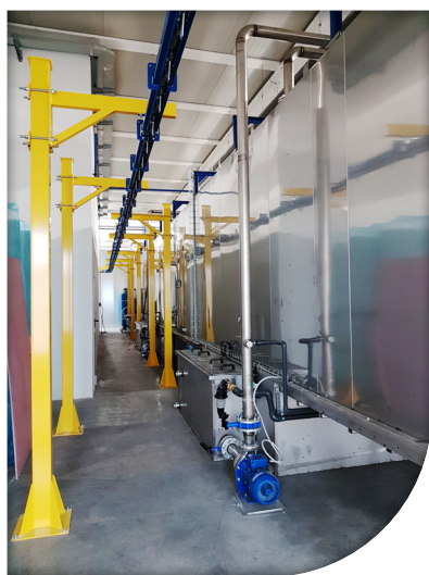
Side view of a 5-stage pretreatment tunnel
