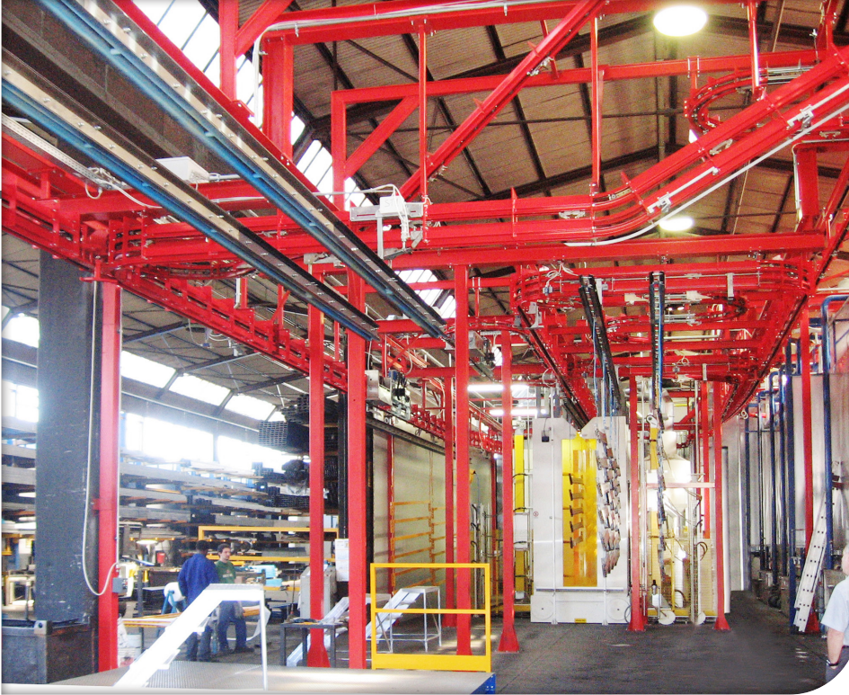
A coating plant for shelving systems with an overhead power & free conveyor
